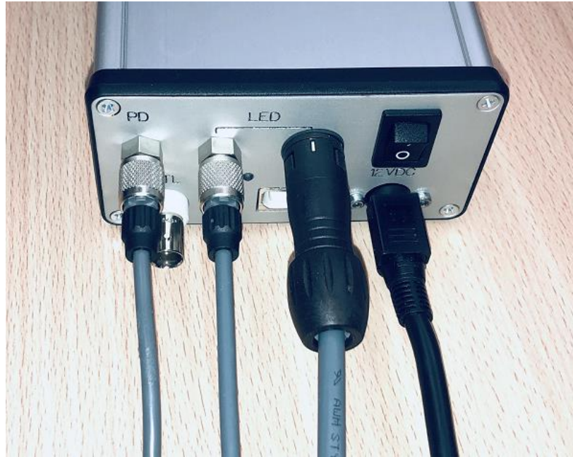
Figure 5a: Cable connections on the back panel of the UHPTLCC-USB-STBL current controller
