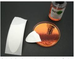
2. Apply the tab to an edge and press down firmly. You can use a piece of a peel tab as in the photo.
