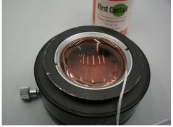
floss down and add a few drops of polymer to "glue" down. Do not put floss directly on optic then apply polymer, it can leave an imprint when removed.
