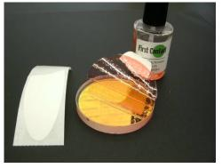
3. Carefully lift the edge of the film with the tab, once the polymer starts to lift it will peel very easy.
