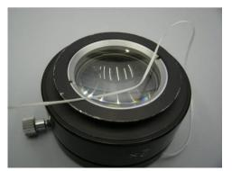
1. An example of an optic recessed in a mount. Floss is used to create a "handle" to remove dried polymer.
