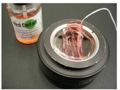
2. Apply polymer, allow to dry a few minutes, place 3. Allow to dry until there is no solvent smell, then carefully pull the exposed end of floss, once the polymer starts to lift it will easily peel out of the cavity.
