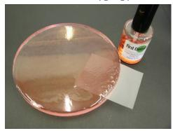
1. Apply polymer, allow to dry a few minutes, place mesh down and add a few drops of polymer over mesh to "glue" down. Do not put mesh directly on optic then apply polymer, it can leave a mesh imprint on the optic when the dried polymer is removed.
